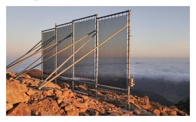
Water passes through nets, condenses on the material, and falls into a storage trough. I'm happy to explain the technical aspects of this at some point - but the punchline is that, with no additional inputs of energy or significant environmental damage, Amazigh families now have as much clean water as they need piped directly into their homes.
